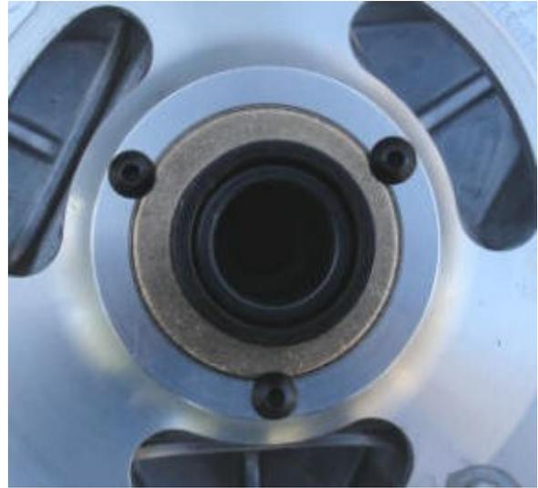
Another advantage of the 911 Response clutch cover is we're replacing a cheapo cast cover with a billet machined cover that is a full-circle instead of being triangular like the OEM ones. The 911 cover is thicker, stiffer and stronger, helping to provide rigidity to the entire clutch assembly. The strong cover frames the towers to keep them from spreading and flexing, especially with big power engines.
