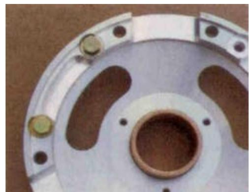
last longer as well. You will very likely never need to replace the cover bushing again. AND you also get Thunder Product's external sheave adjuster so you can adjust the moveable sheave and set the belt side clearance, instead of having to tear the clutch apart or install a new drive belt when it starts to narrow. This is a sweet package.
